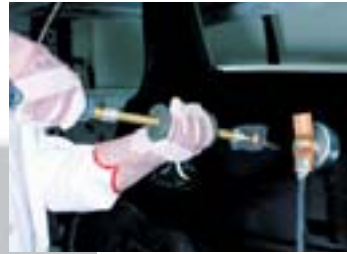
Spot hammer welding
