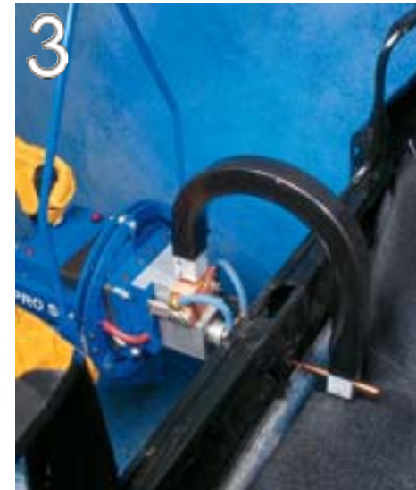
As you swing the head back it will automatically stop at its memory lock position to assure that the tips are perfectly aligned before welding.
