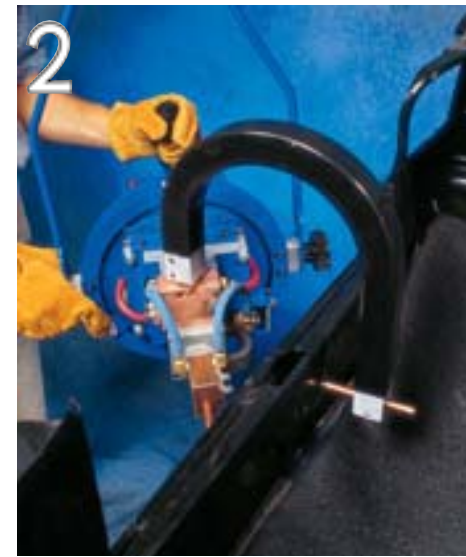
Simply swing the head to make the opening between the tips wider, and lower it down.
